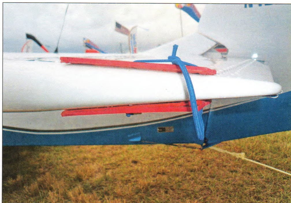
Above: Elevator control lock made from two pieces of plywood and a bungee cord.
